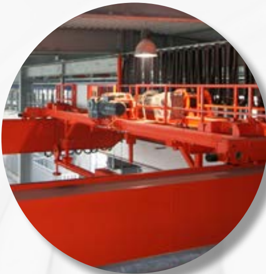
1. The crane trolley in the galvanizing plant receives and sends data via DATAEAGLE slave.
